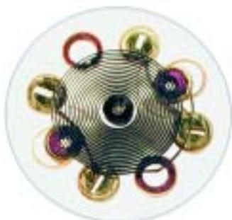
2. At 2 and 8 o'clock, in this 'ultrafine compensation' balance, tantalum discs are attached to curved strips which will move them inward when temperature rises, providing inertia reduction when required.
