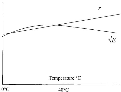
1. The relationship of balance wheel radius,  $r$ , and spring elasticity,  $\sqrt{E}$ , with temperature change. Spring alloys whose anomalous behaviour provides a fairly stable relationship at ambient temperatures are chosen. The vertical scales have been adjusted to emphasise the relationship between  $\sqrt{E}$  and  $r$ .
