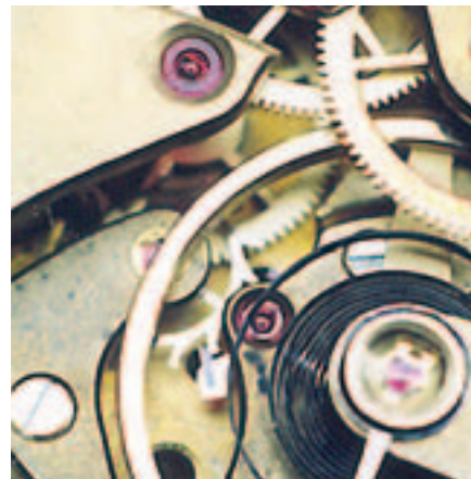
7. High quality deck watch fitted with the author's carbon composite balance spring.
