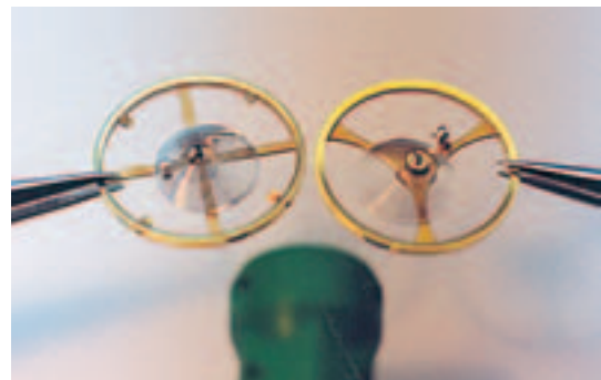
4. Best chronometer and standard balance springs under the influence of a magnet.
