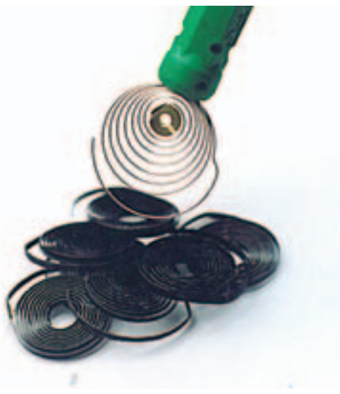
5. Continuous Carbon fibre composite balance springs (black) made by the author, with a standard ferro-nickel spring, in the presence of a magnetic field.
