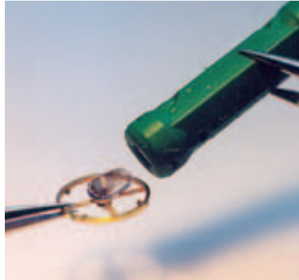
1. A current high-grade COSC-rated balance and spring in the presence of a child's toy magnet.
